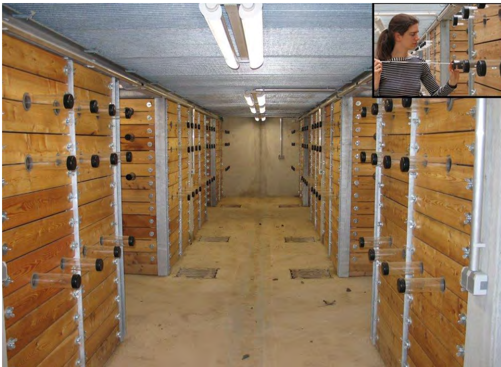
The Göttingen Rhizolab with minirhizotron access tubes
