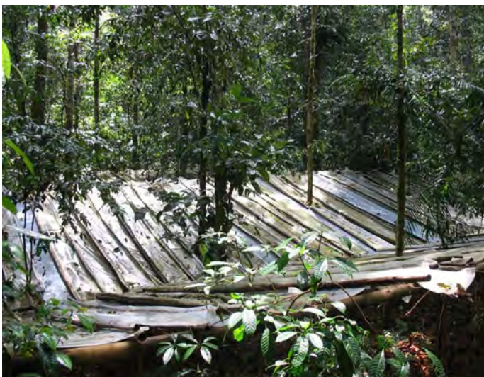
Sulawesi Throughfall Exclusion Experiment (Indonesia) for simulating drought in a tropical rainforest
