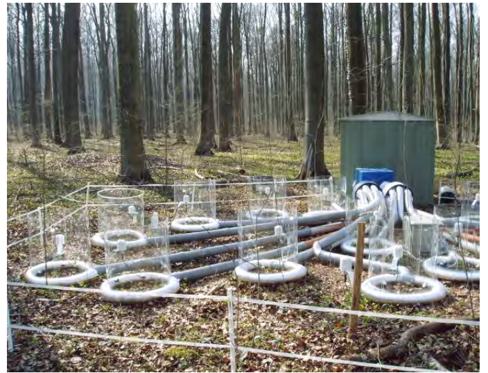
Air humidity manipulation facility on the forest floor
