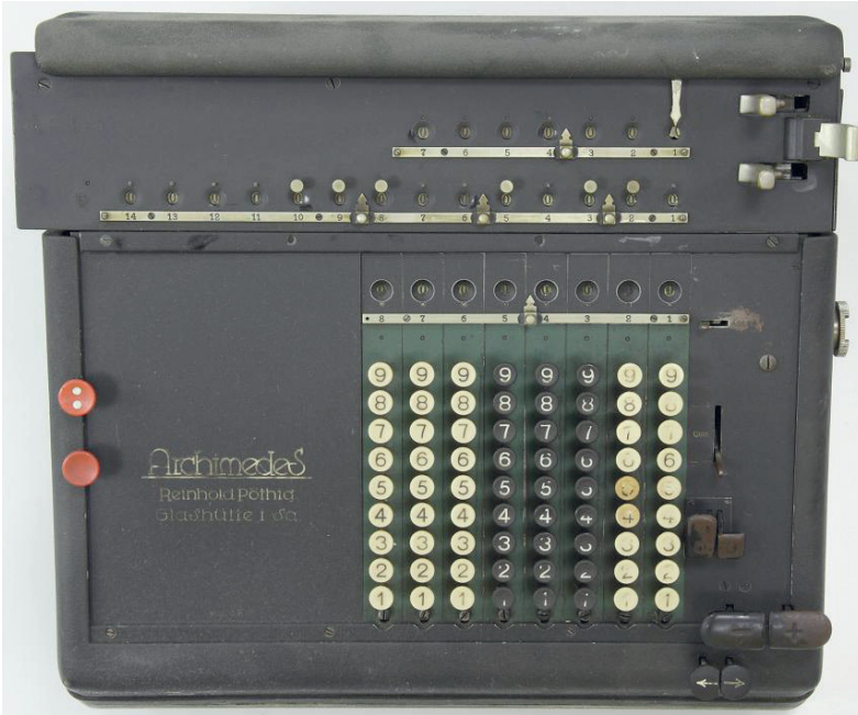
Archimedes-GER. Stepped drum four function electromechanical calculator, 1932
