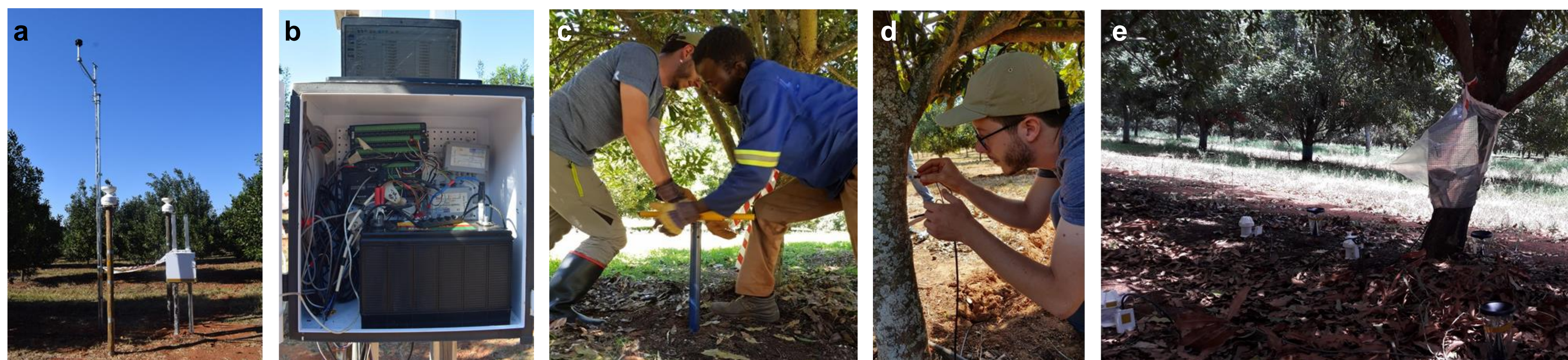
(a) Weather station at Maclands; (b) datalogger, battery and power boxes; (c) taking soil samples for the analysis of soil properties; (d) installing sap flow sensors; (e) combined soil and tree sensors for detailed monitoring of water relations in macadamia orchards (pictures by Bringhenti, T.)
