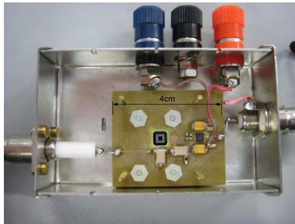
Figure 5.8: Circuit for TCT measurements laid out on a PCB and placed inside a metal box for shielding. This setup is used in conjunction with the pulsed laser diode.
